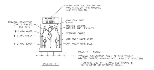
EST STATION INSTALLATION IN MANHOLE
