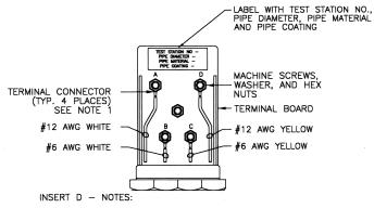
1. TERMINAL CONNECTORS SHALL BE RING TONGUE, BRAZED, COPPER, NON-INSULATED WITH X" STUD SIZE - FOR WIRE SIZE 14-10 AWG, USE THOMAS & BETTS 54101 OR APPROVED EQUAL.
