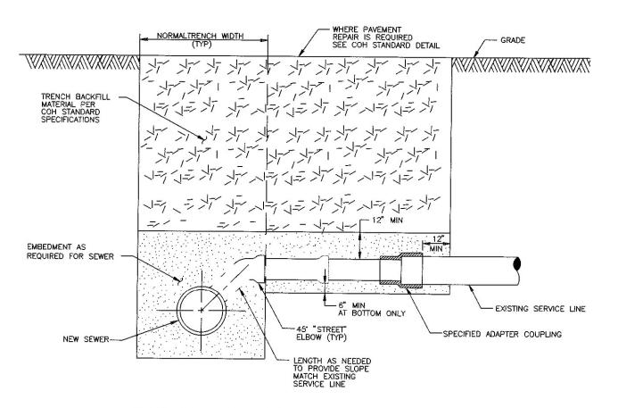
CROSS—SECTION OF SEWER AT SERVICE CONNECTION
